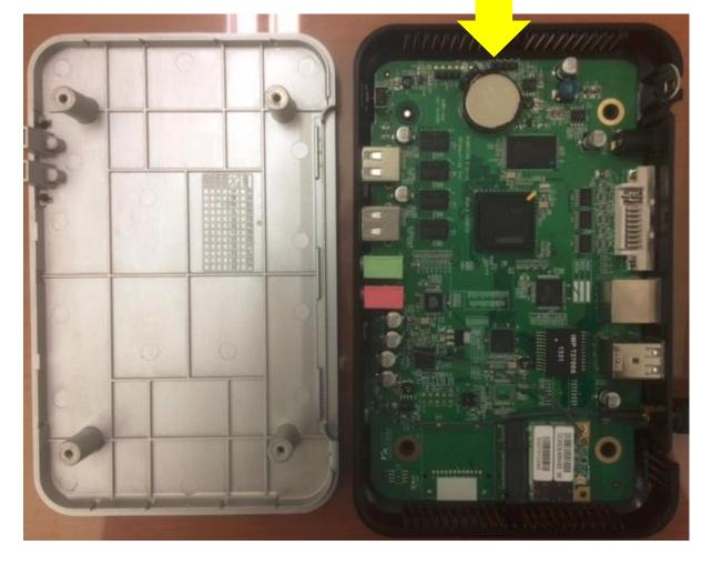
• Step2: remove the failed coin battery and replace to new one (Coin battery\_2032 / CR2032, Coin Type Lithium Battery /
