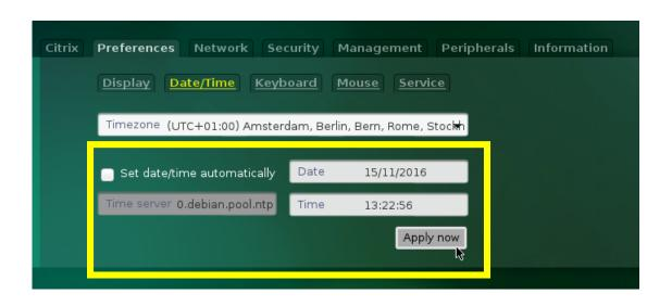
• Step5 : after device time setting, power off/on and done
